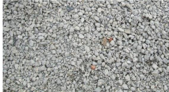
Abb. 23: RC Betonsplitt 2/16 [Mettke]
